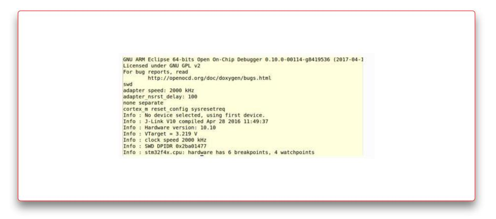
Now, in another terminal, we will open telnet and perform different operations over the JTAG interface. The link <u>here</u> describes in detail the commands for performing different operations including, memory read, write, dump, etc. So, for example to extract the firmware the command is , dump\_image flash\_dump.bin <address> <flash memory length>
