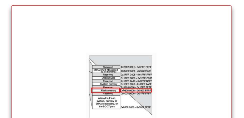
And via the telnet we send the following commands, \* halt \* dump\_image flash\_dump.bin 0x8000000 0x7FFFF \* resume It successfully extracts the firmware from the device, as shown below.
