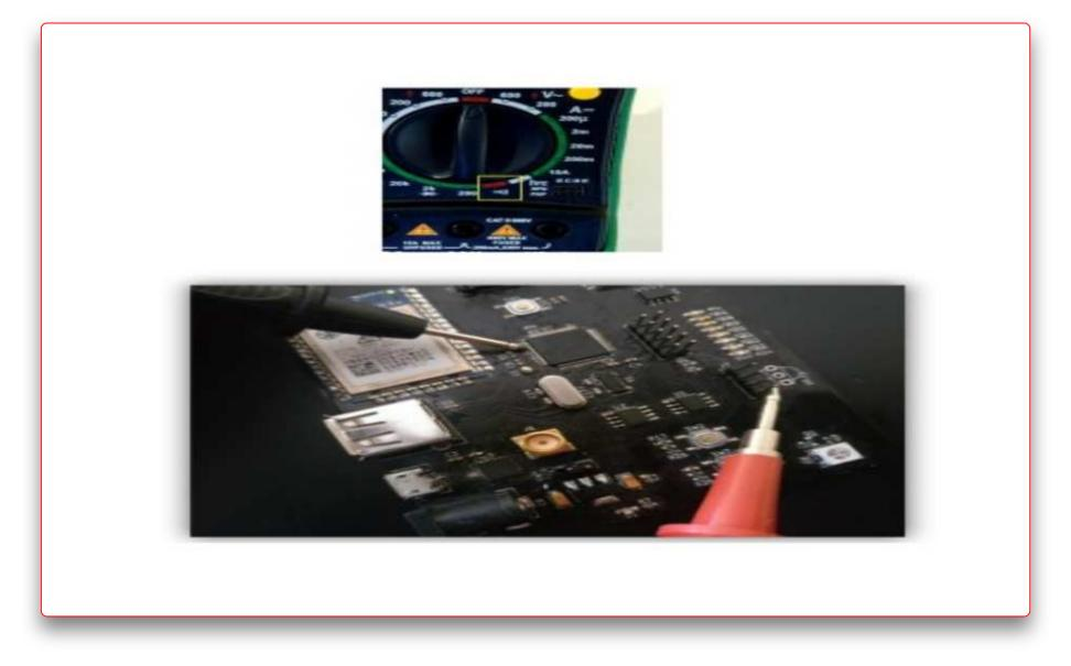
Then, we put one probe on the JTAG port pins on the controller and the other probe on the test points/ headers pins on the PCB suspected to be JTAG port pins. This test is repeated until pins are identified. The procedure for identifying SWD pins is the same. Manual identification is
