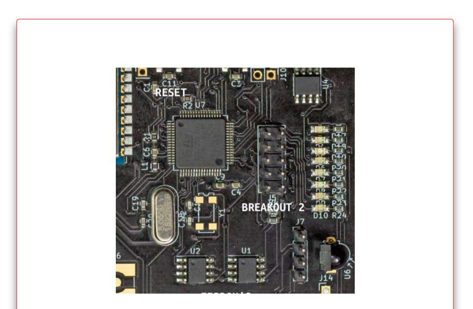
The microcontroller used in the <u>diva board</u> marked as U7 on the PCB is **STM32F411x**, we can search its <u>datasheet</u> for the pins having JTAG/SWD interface connection. The image below shows that section of the datasheet.
