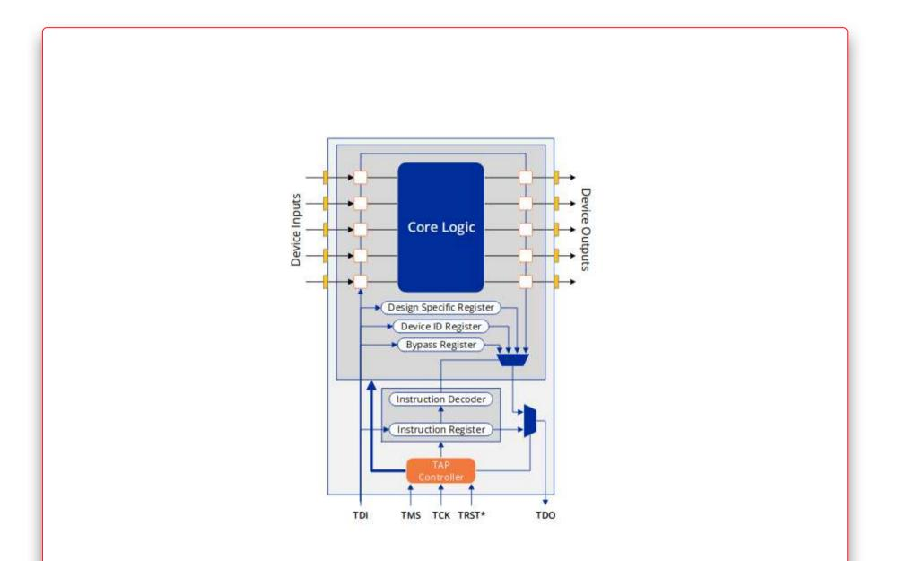
The JTAG chip consists of logic cells or boundary-scan cells that connect the chip to the PCB. These can capture data from pin or core logic signals as well as send data onto pins. These logic cells are accessed through a serial test data input (TDI) and test data output (TDO) interface. The test controller's primary interface that provides access to the logic is the Test Access Port (TAP), consisting of 4 required signals and an optional reset signal.
