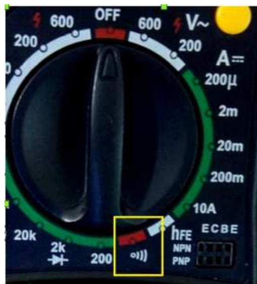
Then, we put one probe on the UART port pins on the controller and the other probe on the test points/ headers pins on the PCB that are suspected to be UART port pins. This test is repeated until pins are identified. Vcc and Ground pins can also be identified similarly.
