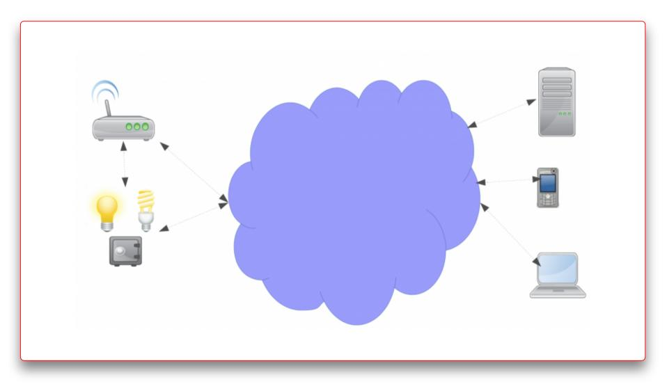
We can also have geographically spread sensor networks that can communicate with/are connected to each other via traditional networks by the IoT Gateways as shown below.
