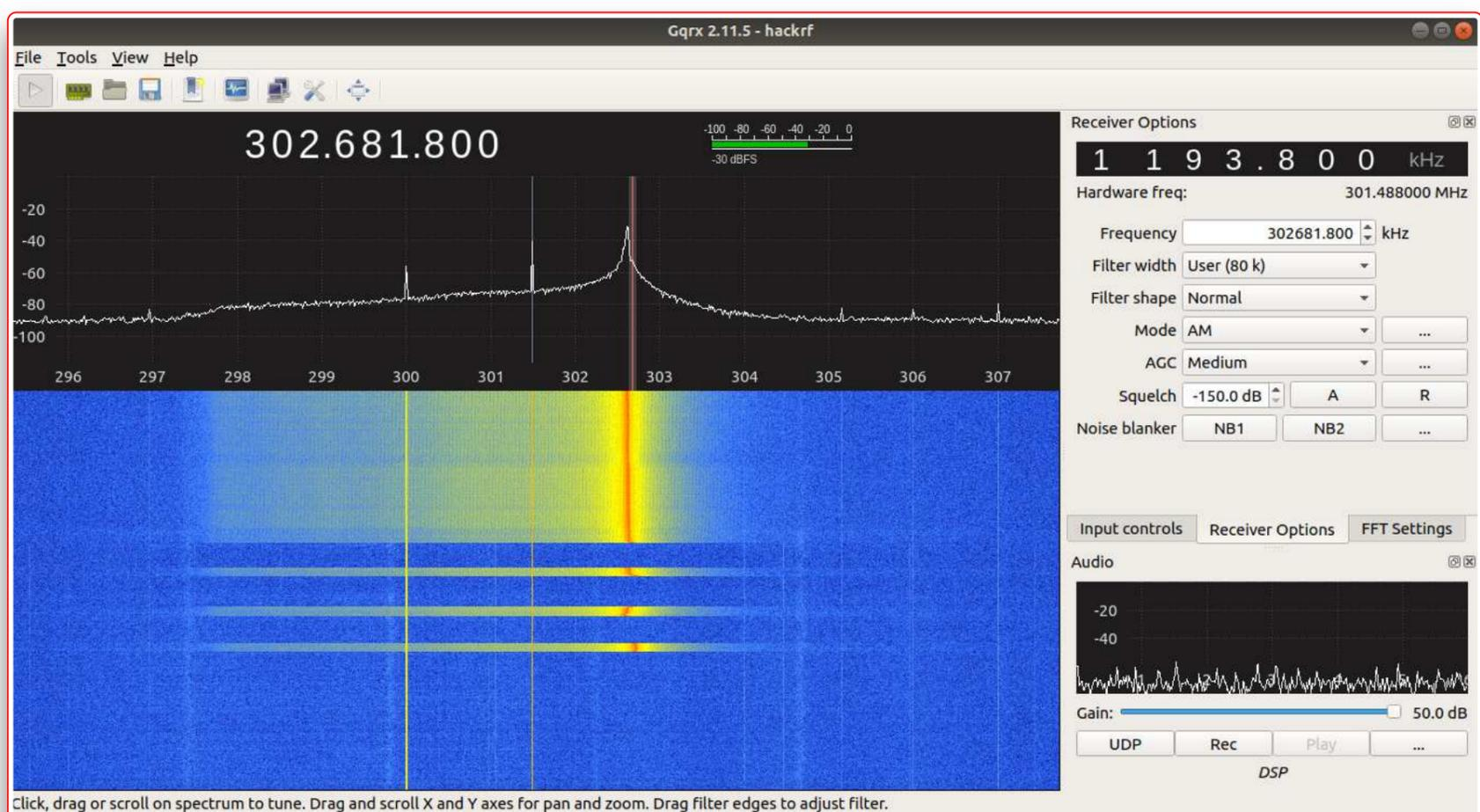
In our case, we used GQRX for this step. We observed the peak at 302MHz, which is a little unusual for any operating device.
