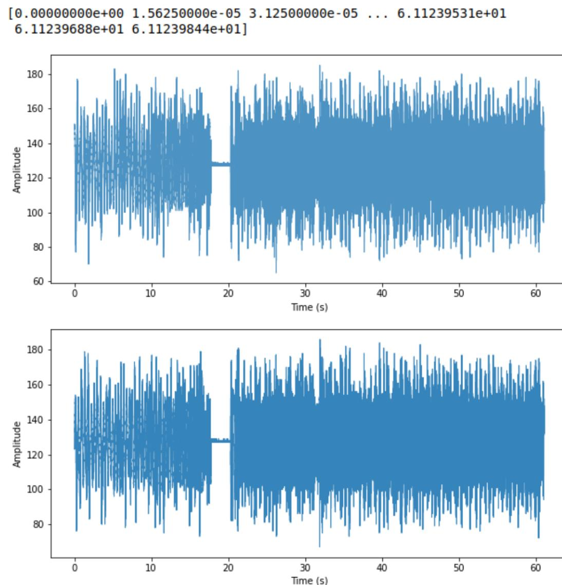
The upper plot is for Inphase channel and the lower is for Quadrature channel
