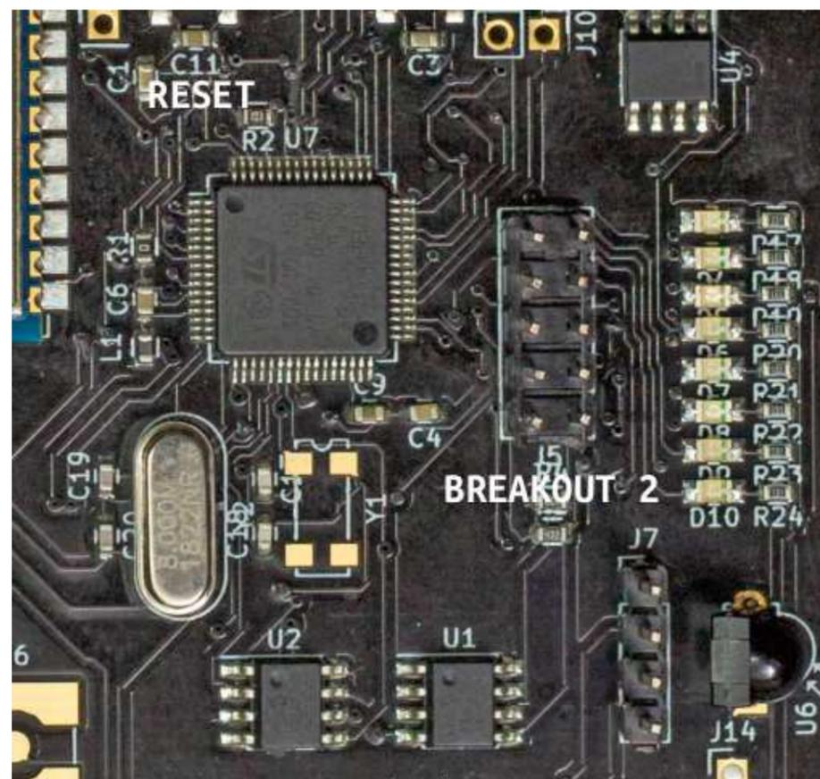
The microcontroller used in the diva board marked as U7 on the PCB is **STM32F411x**, we can search its datasheet for the pins having JTAG/SWD interface connection. The image below shows that section of the datasheet.
