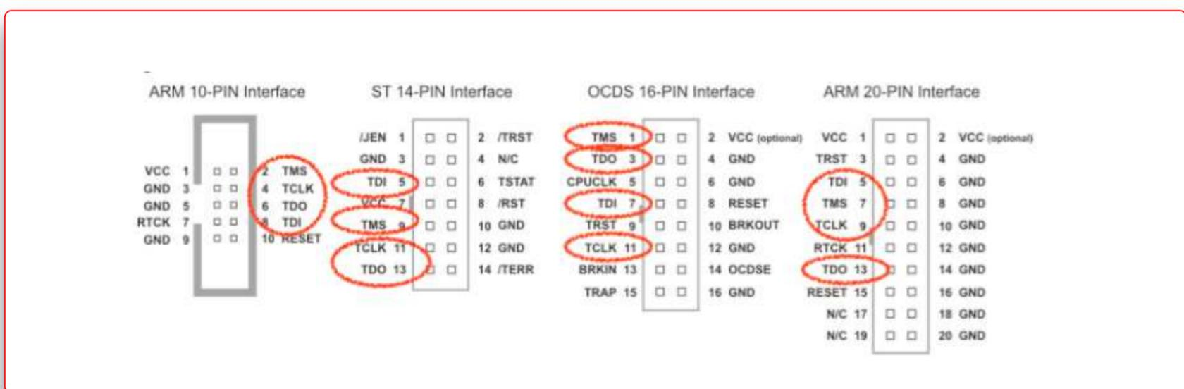
For communicating with the device via the JTAG interface, we would have to identify the 4 JTAG signals TCK, TMS, TDI, and TDO that communicate with the JTAG chip state machine via TAP. It is also possible to communicate with more than one JTAG chips by connecting them in daisy chain as shown in the image below (Source - [Wikipedia](#))
