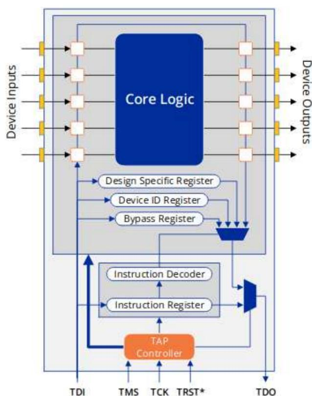
The JTAG chip consists of logic cells or boundary-scan cells that connect the chip to the PCB. These can capture data from pin or core logic signals as well as send data onto pins. These logic cells are accessed through a serial test data input (TDI) and test data output (TDO) interface. The test controller's primary interface that provides access to the logic is the Test Access Port (TAP), consisting of 4 required signals and an optional reset signal.
