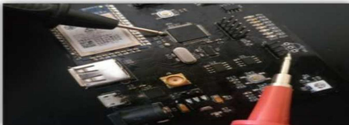
Then, we put one probe on the JTAG port pins on the controller and the other probe on the test points/ headers pins on the PCB suspected to be JTAG port pins. This test is repeated until pins are identified. The procedure for identifying SWD pins is the same. Manual identification is
