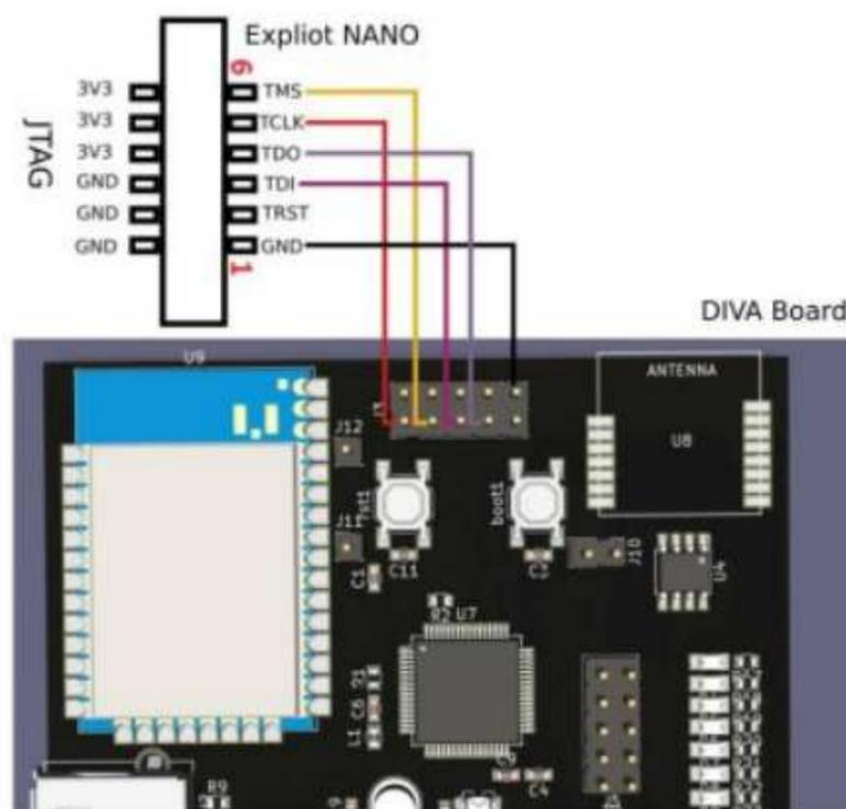
Now, to communicate with the JTAG interface, we need to launch the **Openocd**, `$ openocd -f exploit_nano_jtag.cfg`.
